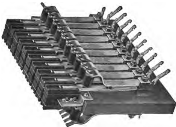
FIG. 109.—Switchboard protective apparatus, heat coils and lightning arresters.
